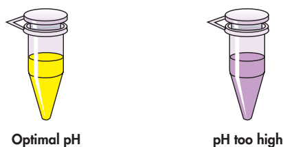
Figure 3. Indicator enables easy checking of the optimal pH. Indicator dye in solubilization and binding Buffers QG and PB identifies optimal pH for DNA binding.
