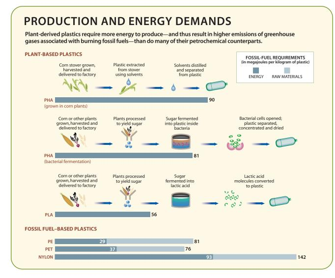
first approach, which turns sugar from corn and other plants into a plastic called polylactide (PLA). Microorganisms transform the sugar into lactic acid, and another step chemically links the molecules of lactic acid into chains of plastic with attributes similar to polyethylene terephthalate (PET), a petrochemical plastic used in soda bottles and clothing fibers.
