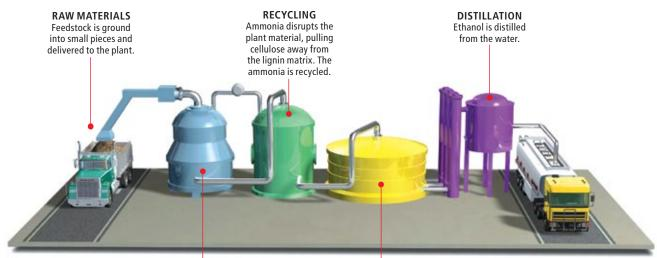
**PRESSURE COOKING** Feedstock mixes with ammonia, a strong base, under heat and pressure. FERMENTATION Treated cellulose is broken down into sugars by enzymes and then fermented into ethanol.
